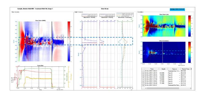
Dashboard of interactive software for Far-Field Strain (FFS) data processing, frac hitsand frac hit corridor (FHC) picking. Left top: strain data colored by red-blue scale presents tension-compression; Left bottom: pumping data; Center: strain curves red=tension, blue=compression for bothinstanteous and cumulative strain; Right top/middle: strain heat map; Right bottom: frac hits picking data.
