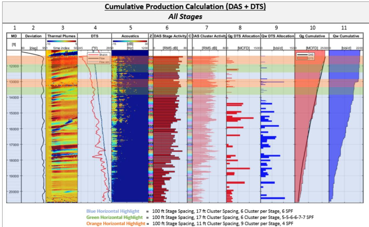
All stages DAS and DTS composite production allocation for 100% open choke.
