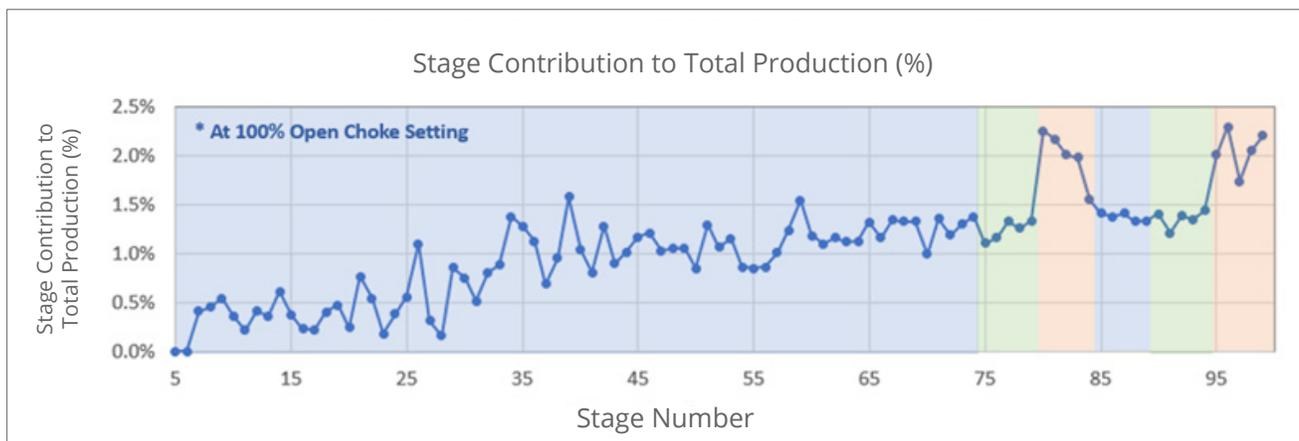
Stage contribution to total production (%) using DAS allocation data highlighted by design. Toe-side stages contribute much less toward total production compared to the heel.
