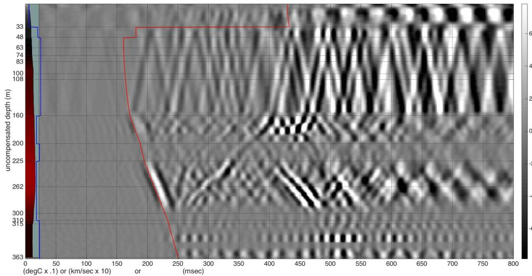
ULTIMA DTS temperature profile and iDAS active source seismic data from the downhole installation at Brady’s Hot Springs. The DTS temperature profile collected during a thermal recovery period indicates that the rock formation has cooled below 262 m due to power plant operations. iDAS active seismic data showcasing cable coupling and P and S wave signal.
