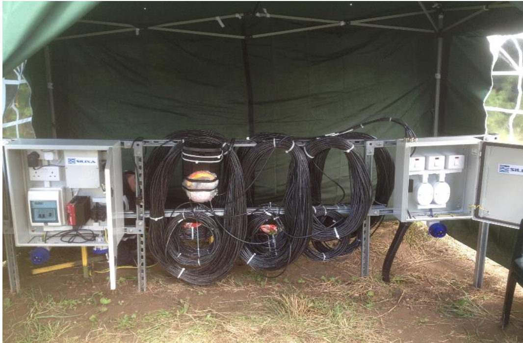
Figure 3: Active and passive DTS monitoring system for soil heat and moisture dynamics.
