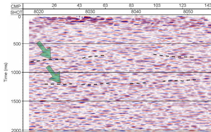
**Figure 15.** Band-pass-filtered (5-16-45-50 Hz) stacked time section, with post-stack mix and AGC for visualisation purposes, of the SmartSolo® data (vertical component). The green arrows and the dashed lines indicate the expected reservoirs in two-way travel time.
