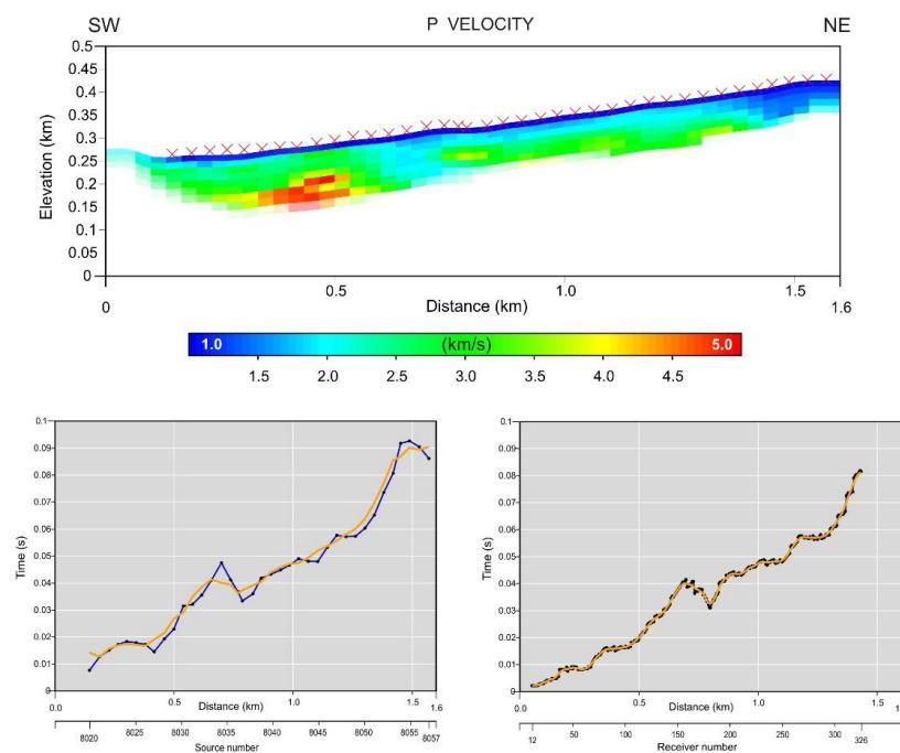
**Figure 9.** Compressional velocity section obtained from inversion of first arrivals (top), using the simultaneous iterative reconstruction technique (SIRT) algorithm [52]. Red crosses are the shot points. The bottom panels show the smoothed applied static corrections (yellow solid line) and punctual static corrections (blue) for sources (left) and receivers (right), respectively.
