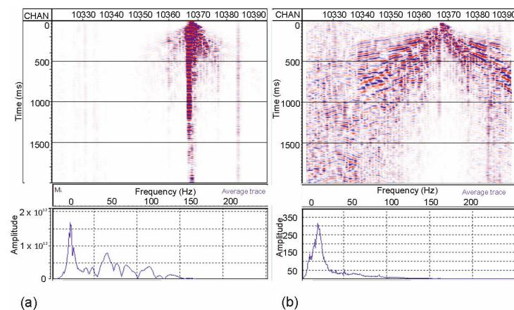
**Figure 12.** SmartSolo®’s common-shot (**top**) for the common-shot gather 8041 before (**a**) and after (**b**) balancing. The blue lines in the bottom of the figures are the corresponding frequency spectra.
