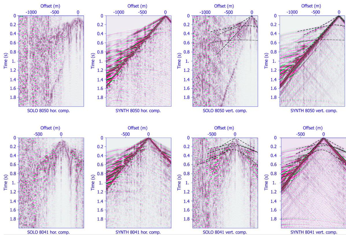
**Figure 7.** Common-shot gathers: comparison between the horizontal and vertical components of the SmartSolo® geophones and the corresponding synthetic particle velocity components for shots 8050 (**top**) and 8041 (**bottom**). Synthetic data are computed using the velocity models of Figure 6a and a vertical point source with a 20 Hz peak frequency. As an example, the dotted lines in the vertical components of the shots highlight the qualitative similar trends of selected events.
