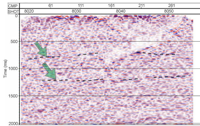
**Figure 14.** Band-pass-filtered (5-16-45-50 Hz) HWC DAS stacked time section after post-stack mix and AGC for visualisation purposes only. The green arrows and the dashed lines indicate the expected reservoirs in two-way travel time (TWT).
