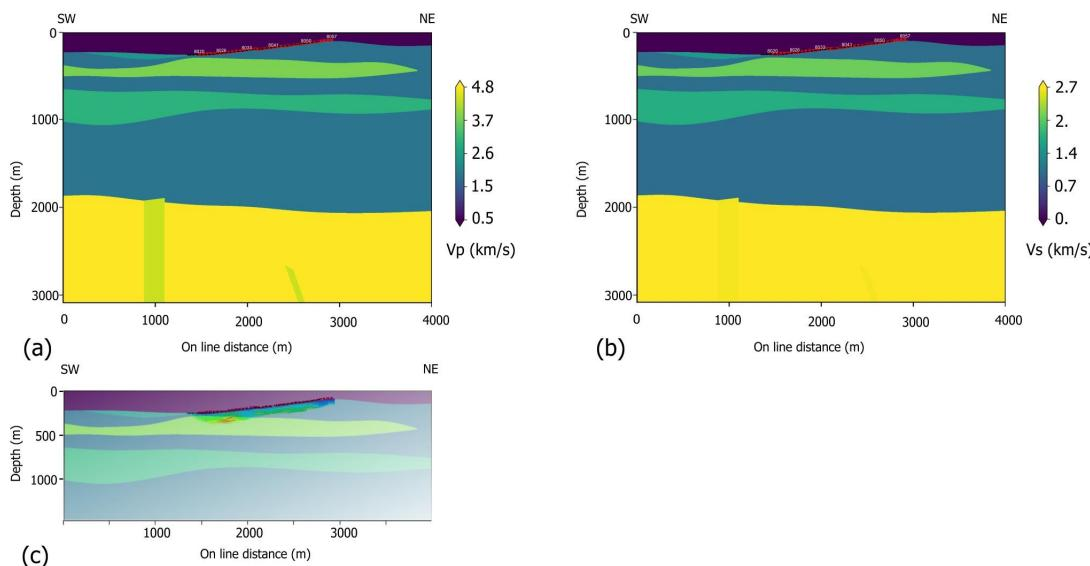
**Figure 6.** SW-NE-oriented models: (a) final compressional velocity model; (b) shear velocity model updated using the results from the laboratory transmission experiments. (c) A blow-up of the shallower part of the model (up to about 1500 m depth) in (a) with the superimposed result of the first-break tomography. The velocity scale is the same as in (a), but a transparency has been applied to highlight the superimposed result.
