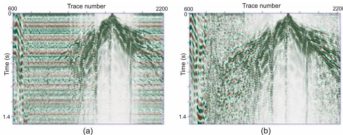
**Figure 8.** (a) Common-shot gather 8041 from HWC DAS recordings affected by optical noise (horizontal stripes). (b) The same shot gather after optical noise removal and signal recovery. Data are not filtered.
