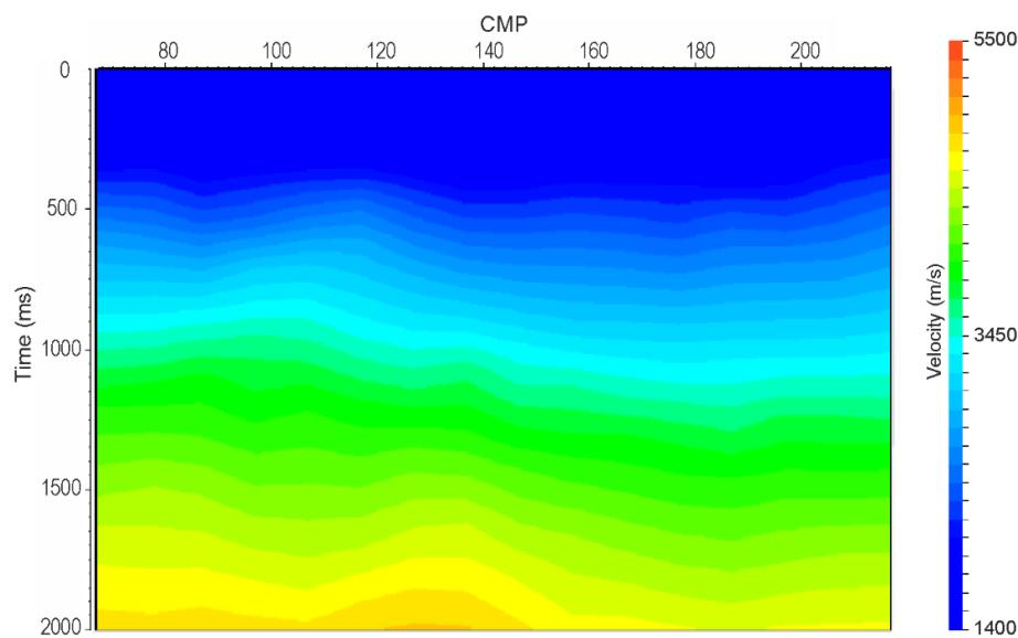
**Figure 11.** 2D stacking velocity section calculated from the HWC DAS dataset.
