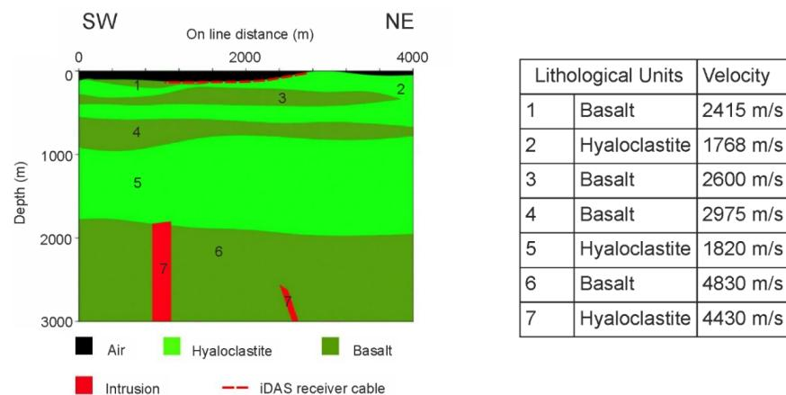
**Figure 5.** Hellisheiði field site geological model used for seismic simulations where the topography was updated according to the elevation of the receivers. The main lithologies are indicated in the legend and the receiver cable position is marked with a red dashed line. The table lists the average velocities for the layers.
