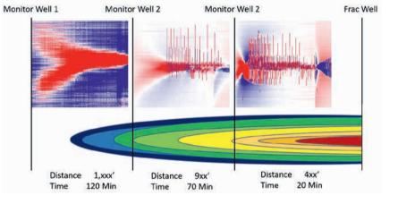
Figure 7 Monitoring the poroelastic effect and frac hits passing through three fibre locations.
