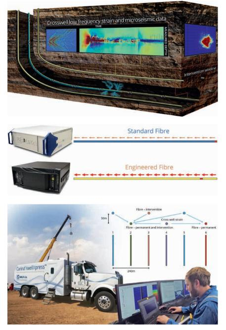
Figure 2 Real-time Hydraulic Fracture Monitoring (HFM) in multiple wells using engineered fibre deployed permanently and on a wireline intervention cable.
