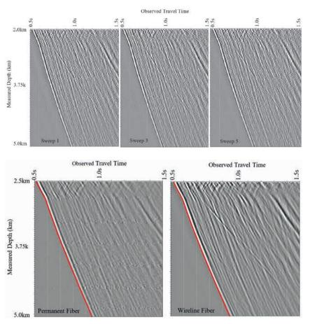
Figure 10 Raw VSP sweeps using intervention cable in a high deviated well.
