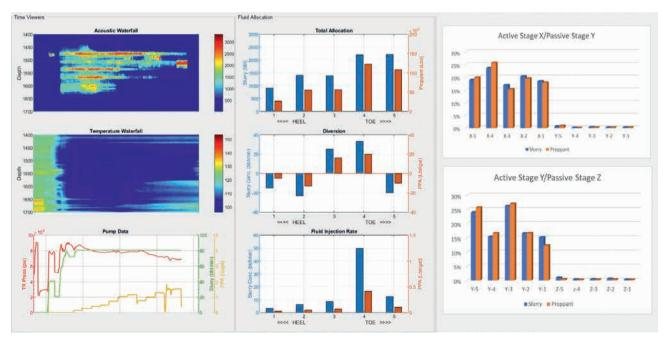
Figure 1 Distributed Acoustic Sensor (DAS) and Distributed Temperature Sensor (DTS) data recorded in real time on a permanent fibre installed on to the outside of the casing to analyse the fluid allocations per cluster.
