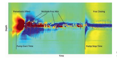
Figure 5 Colour map of the crosswell strain at depth versus time (600 m-wide over few hours).
