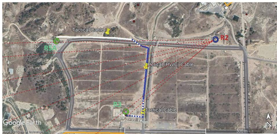
Fig. 7. Location of the planned CO<sub>2</sub> injection well R2 and the two monitoring wells R3 and R5A where the downhole Constellation fibres will be installed at the Zorlu Energy Kizildere geothermal field. The blue line is the HWC deployment and the white line is the tactical cable joining the two downhole cables and the HWC to the DAS interrogator. The red dashed lines indicate the tracer flow paths from previous tests at the site.
