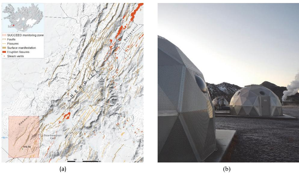
Fig. 4.(a) The Hengill volcanic system and the SUCCCEED seismic monitoring zone around the HN-16 CO<sub>2</sub> injection well at the Hellisheiði site marked with a red rectangle (Courtesy of T.A. Thorgeirsson, Reykjavík Energy, 2020), (b) the Hellisheiði site brine and CO<sub>2</sub> injection wellfield.
