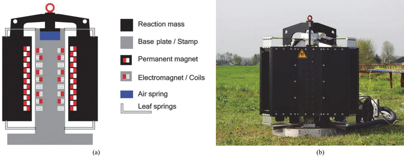
Fig. 2. (a) A 2D sketch showing the different components of the original prototype LSM vibrator, (b) Prototype vibrator deployed in the field [10].
