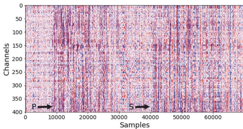
Fig. 6. A recording on the surface HWC of a M3.3 earthquake on 23 July 2020 with an epicentre approximately 100km from the Hellisheiði power plant. The time of P- and S-wave arrivals are indicated [15].
