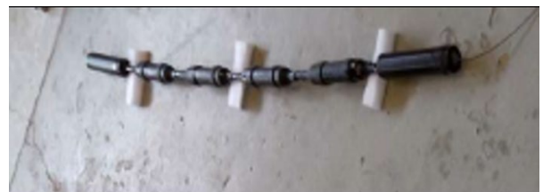
Fig. 4. The picture shows the first small array with four hydrophones built in a semi-automated way.
