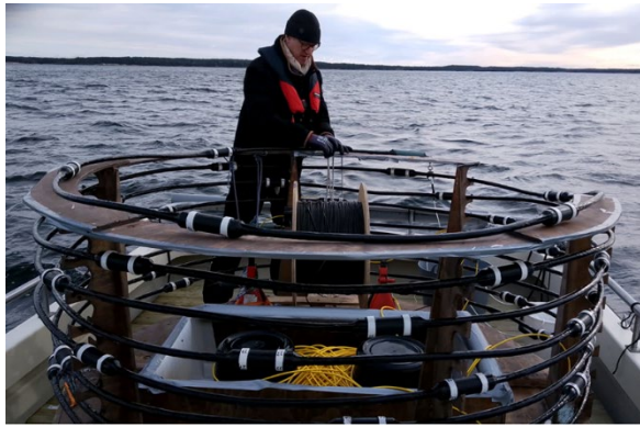
Fig. 5. Carousell to deploy more than 3000 m of fiber optic cable including 48 fiber optic hydrophone elements.
