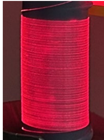
Fig. 1. The picture shows a high sensitivity Coiled Fiber Optic Hydrophone. The short size of the hydrophones makes them omnidirectional. The active part is about 5 cm long.
